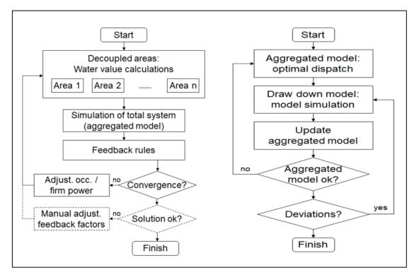
Figure 2.3 Flowchart of EMPS (left) and EOPS (right) model(33)
