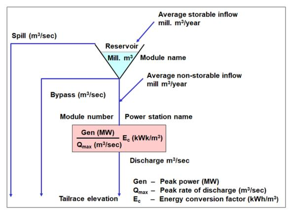
Figure 4.5 Model of a hydropower plant in EMPS(33)
