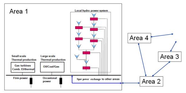
Figure 2.4 Schematic description of an EMPS area(33)
