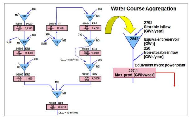
Figure 4.6 Aggregation of hydropower plants(33)
