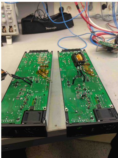
Figure 5.1: The two modules used, shown side by side from the bottom side. The resonant inductor L_r is what sticks out. It is desoldered to be able to attach a current probe. The rest of the resonant tank and the transistors is inside the module.
