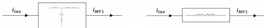
Figure 6.2: Block diagrams of current control with and without C_f as implemented in simulation model
