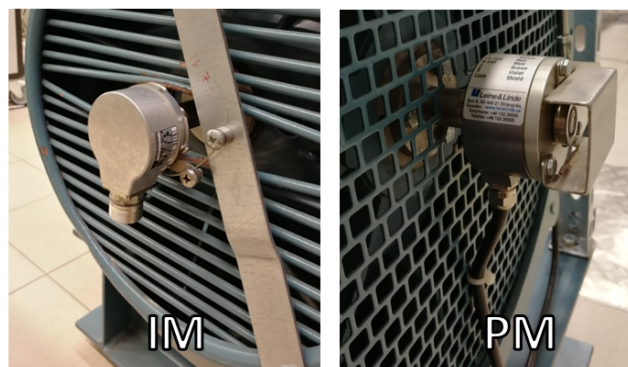
Figure 13.4: Position encoders for induction machines. IM not connected in picture.
