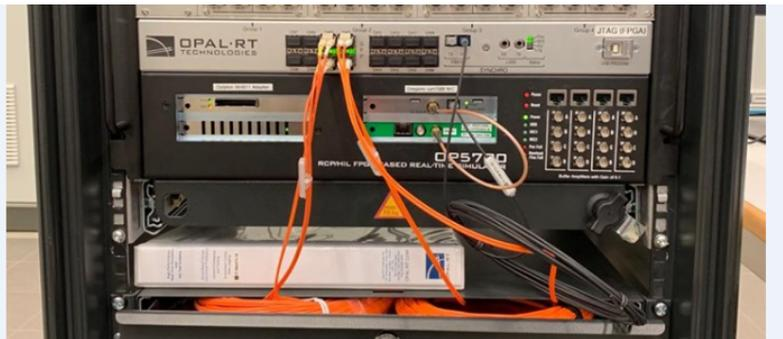
Figure 4.3: Real-time simulation system/Real-time target used for the simulations
