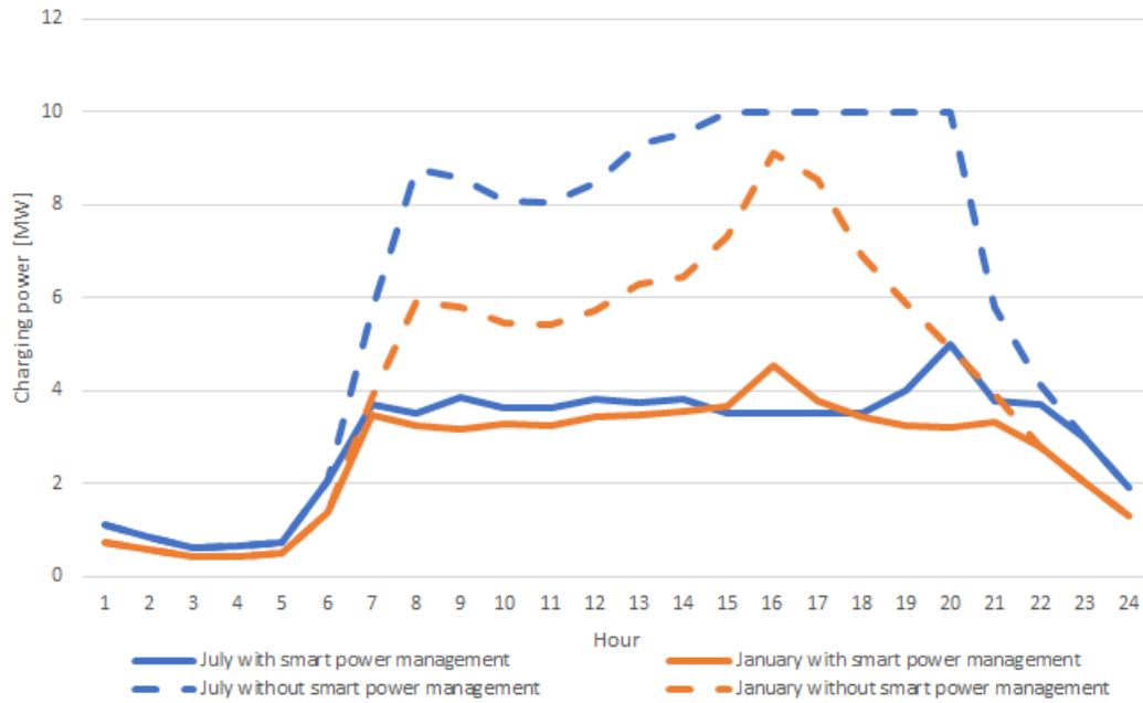
Figure 5.11: Available charging power with and without smart power management for a weekday in January and July in location C
