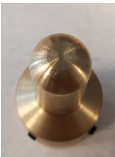
Figure 25: Pin contact used for 152 breakdown test in the setup described in Chapter 4
