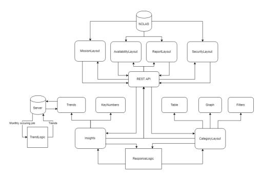
Figure 4.27: Final prototype - structural overview of components and data flow
