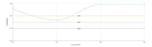
**Figure 4.21:** Final prototype - the process control setting enables three lines that indicate up to three standard deviations of the average.
