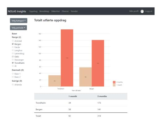
**Figure 4.4:** Prototype II - the operational performance layout showing the number of missions executed at two bases in different periods.
