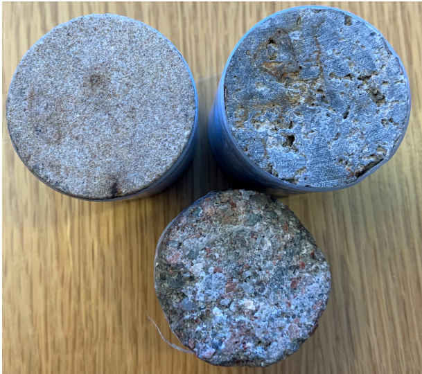
Figure 3.2: Core samples of sandstone, Berea (left), Bentheimer (bottom) and Carbonate (right).
