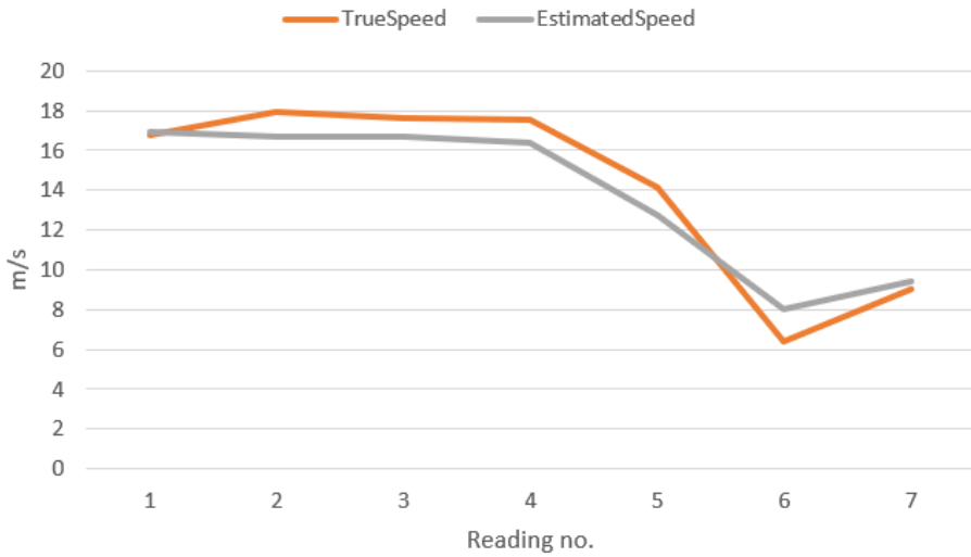
Figure 6.10: Speed analysis 2 - Plot of the true calculated speed and estimated speed of the system
