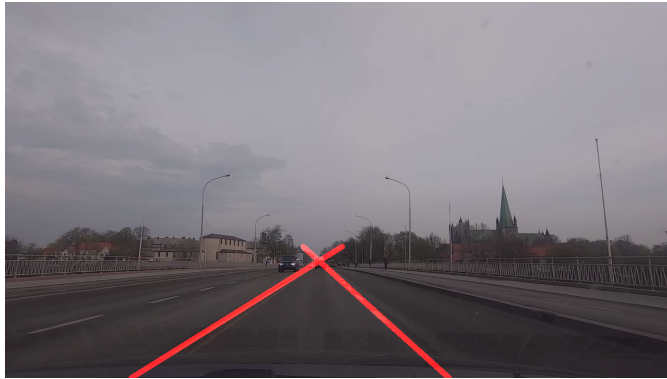
Figure 5.6: Lanes Detected at the Road
