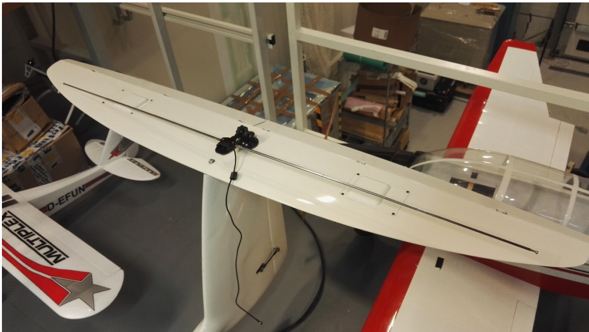
Figure 6.6: VHF antenna mounted on top of the tail wing
