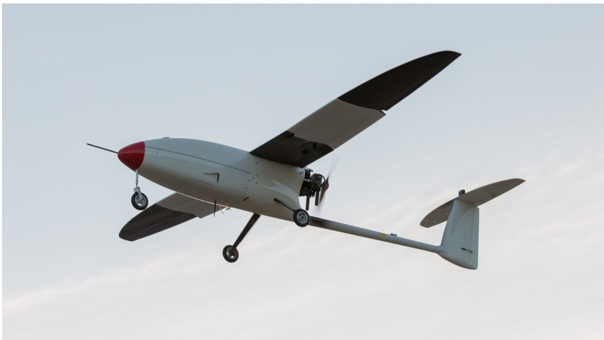
Figure 2.3: ASCs Cruiser 2 UAV in flight (photo by ASC)
