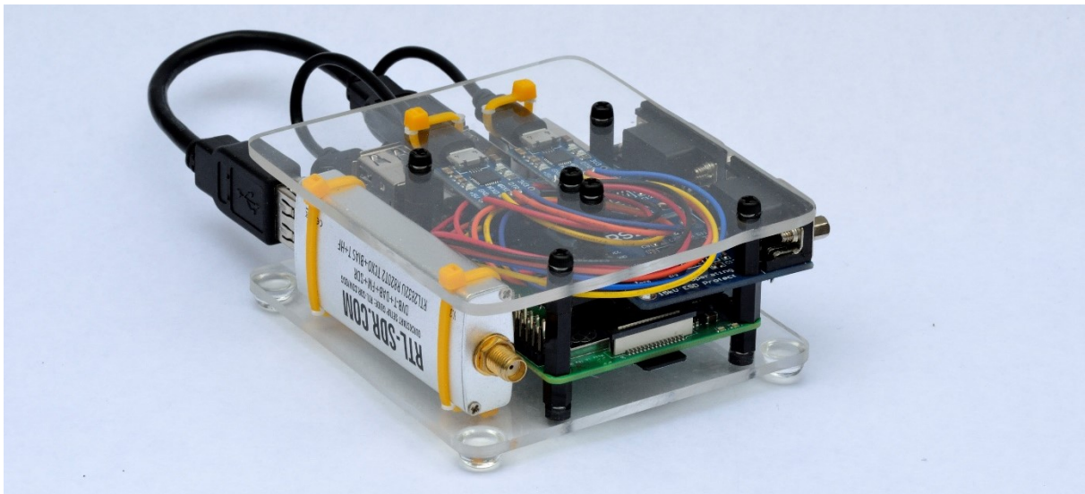
Figure 5.5: The Raspberry Pi 3 Model B+ single board computer, with the serial port modules as well as the SDR.
