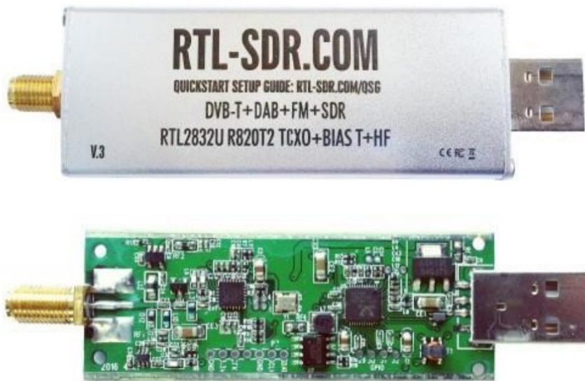
Figure 5.1: The RTL-SDR V.3, an inexpensive, easily available and much used SDR that is well suited for GBAS reception (photo rtl-sdr.com)
