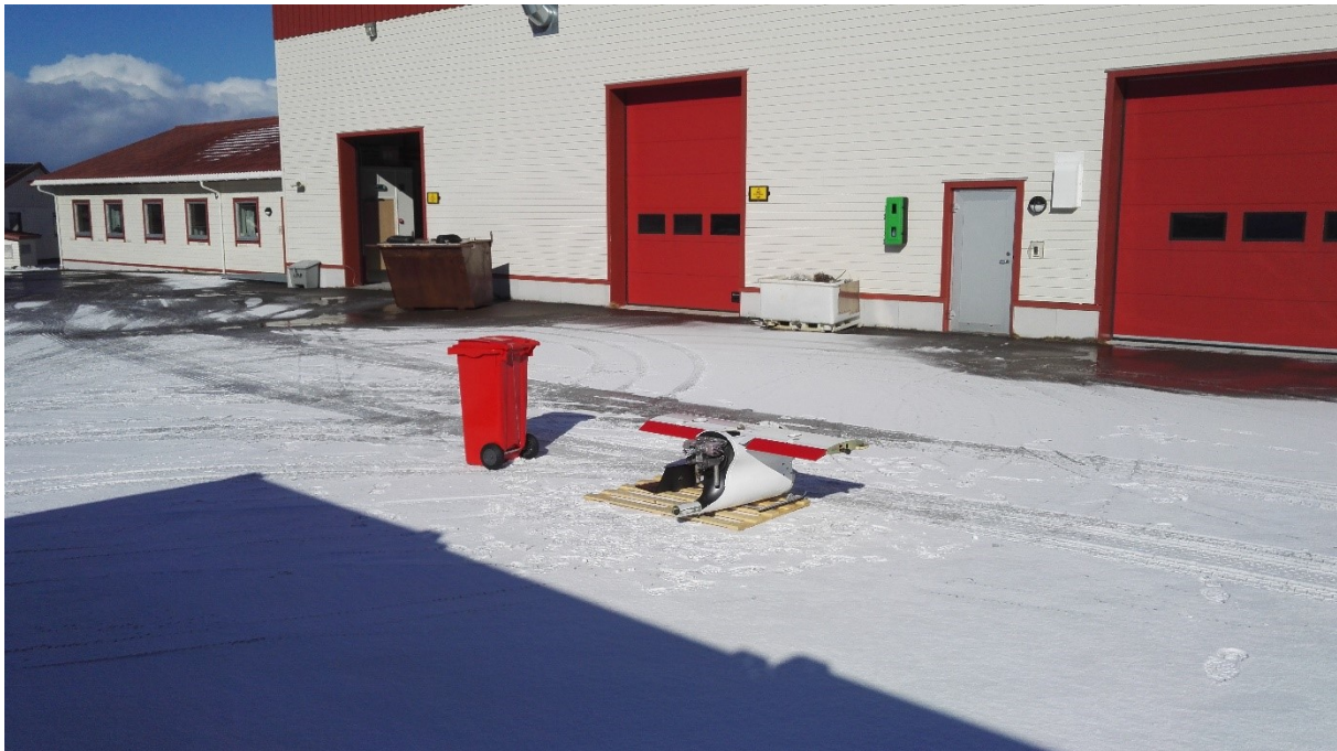
Figure 6.7: Avionics compartment with center-part of wing placed outside in the parking lot at ASC, collecting GPS data.
