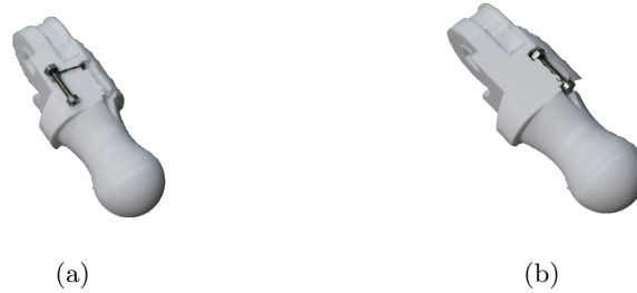
Figure 3.10: First tendon tightening system.
