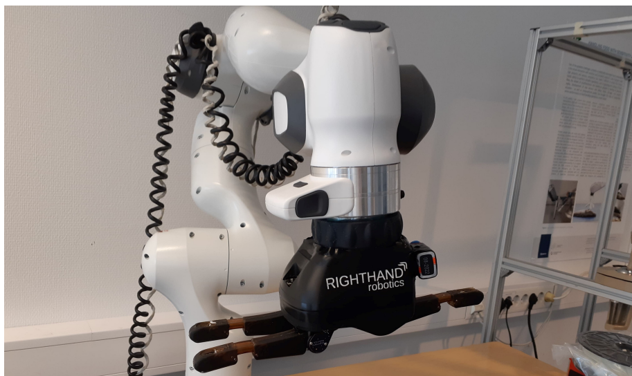
Figure 1.1: Industrial robot arm with Right Hand Robotics REFLEX gripper.
