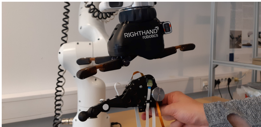
Figure 7.4: Right Hand Robotics' REFLEX and dexterous finger size comparison.
