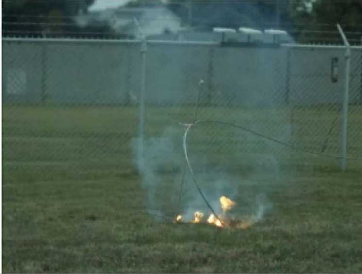
Figure 2.3: High Impedance Fault causing an electric arc [10].
