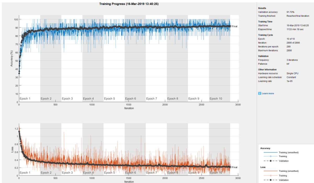
Figure 61: Training progression for network 3. 91,70% validation accuracy. Learning rate 1 \times 10^{-5} . Total of 10 epochs. Elapsed time: 1133 min and 19 sec ( \sim 19 hours) on single CPU.
