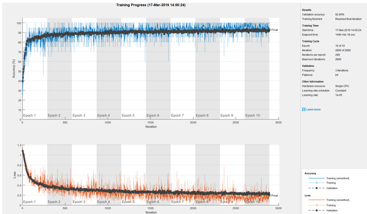
Figure 63: Training progression for network 4. 92,95% validation accuracy. Learning rate 1 \times 10^{-5} . Total of 10 epochs. Elapsed time: 1490 min and 18 sec ( \sim 25 hours) on single CPU.
