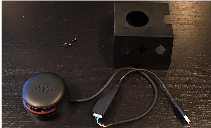
(a) All parts for the LIDAR
