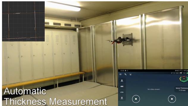
Figure 18.3: Snapshot from the video showing the contact and valid measurement
