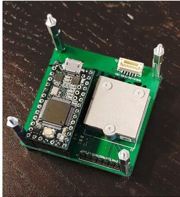
Figure 14.7: The ADIS IMU and the carrier board with the Teensy microcontroller. Designed and developed by Scout DI
