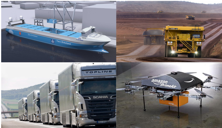
Figure 1.1: Top left: Yara Birkeland, an autonomous container-vessel under development by Kongsberg Maritime, courtesy of Kongsberg Maritime. Top right: Autonomous hauling-trucks, courtesy of Christian Spronge Photography. Bottom left: Four autonomous trucks platooning, courtesy of Scania. Bottom right: Autonomous package delivering drones, courtesy of Amazon.
