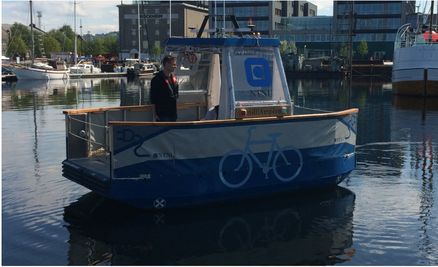
Figure 1.2: The prototype milliAmpere during sea trials. The ferry functions as a platform for development and testing of sensor systems, situational awareness algorithms, COLAV systems and control systems needed for fully autonomous transits. Courtesy of Nicholas Dalhaug.
