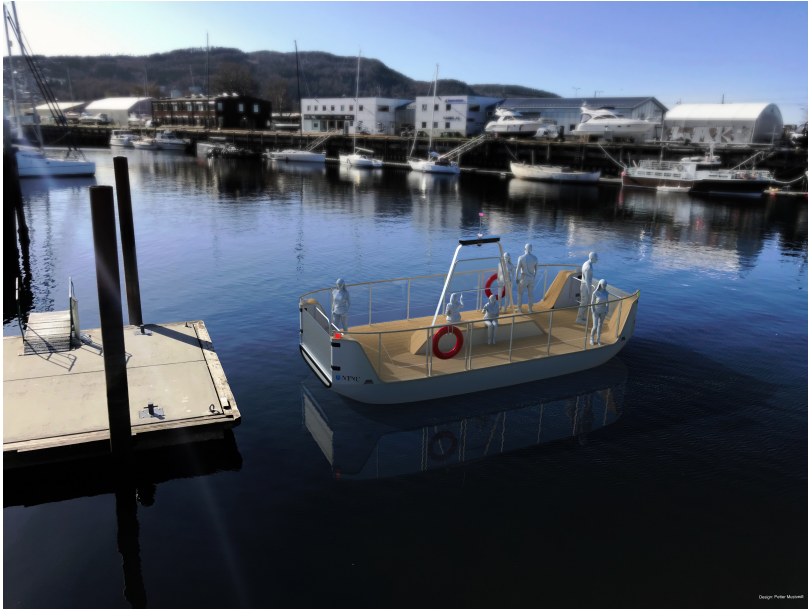
Figure 1.3: Illustration of the full-scale autonomous ferry that is under development at NTNU. Courtesy of Petter Mustvedt, Institute of design, NTNU.
