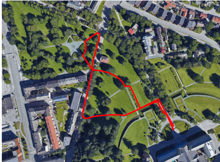
Figure 2: A short walk taken while filming with a cellphone. The small trip features two potential loop closures, and ends where it started
