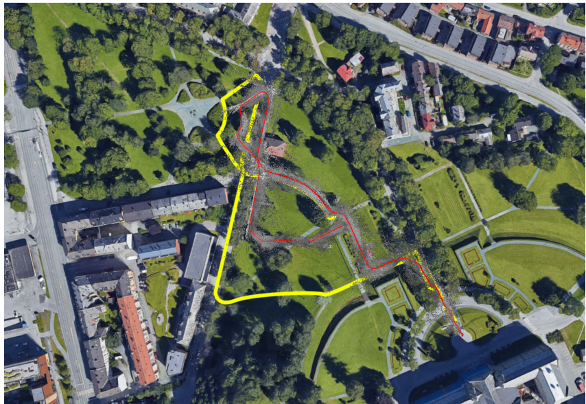
(b) DSO's performance on top of the map of the path taken, showing its large drift in scale
