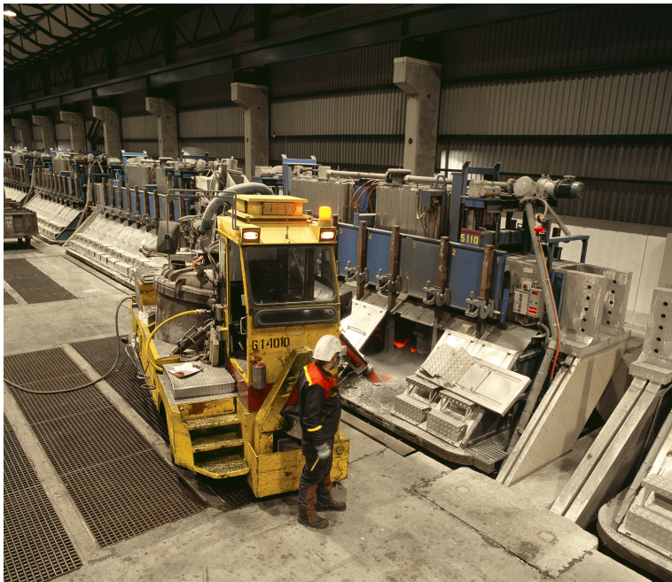
Figure 2.6: Metal tapping by use of specialized vehicle (picture courtesy of Alcoa Mosjøen).
