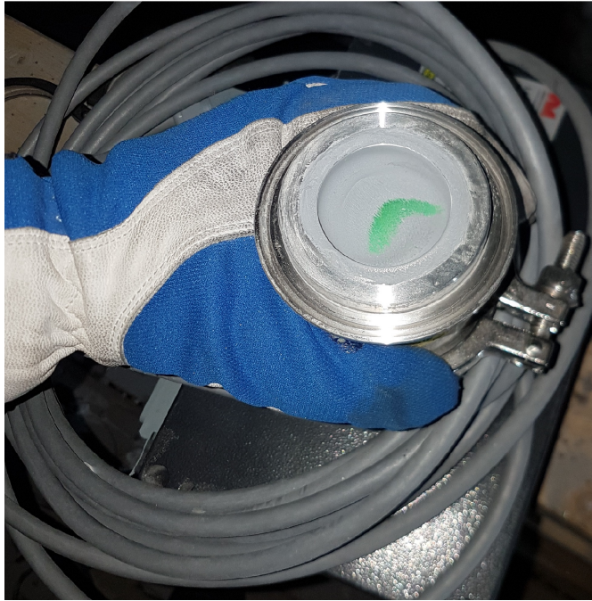
Figure 3.6: Detector optical window before cleaning.
