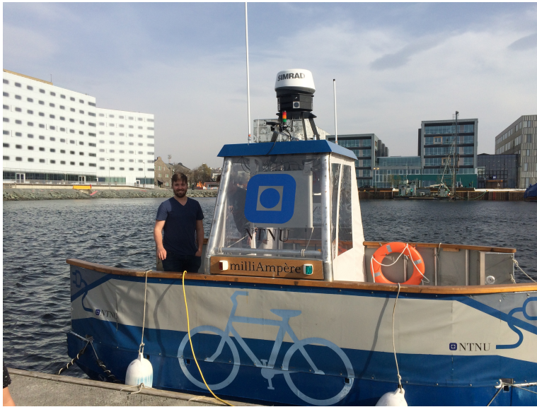
Figure 1: MilliAmpère with the MR sensor rig mounted.
