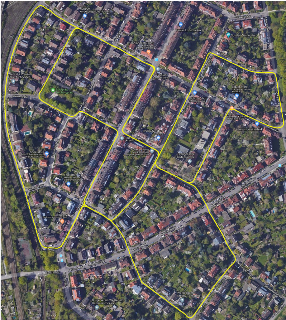
Figure 8.19: Trajectory estimate from SLAM with GNSS measurement every 500 th keyframe plotted over a satellite photo.
