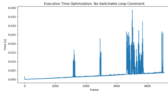
Figure 8.22: Execution time of optimization without the switchable loop constraint. Mean is 2ms, max is 39ms.
