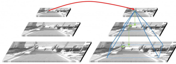
Figure 5.4: Optical flow pyramid: An initial estimate of the optical flow is computed for the image at lowest resolution, and continuously refined through the higher resolution levels down to the original image resulting in the final flow estimate \mathbf{d} .
