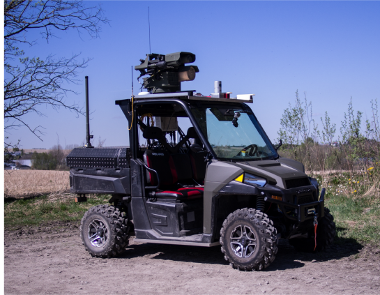
Figure 1.1: Olav, a Polaris Ranger XP 900 EPS is the autonomous platform.
