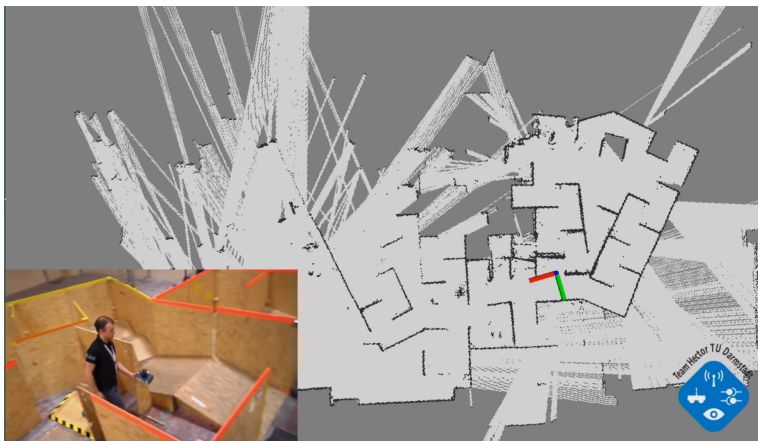
Figure 3.5: Hector SLAM on a handheld mapping device. Ill.: Team Hector Darmstadt/Youtube.
