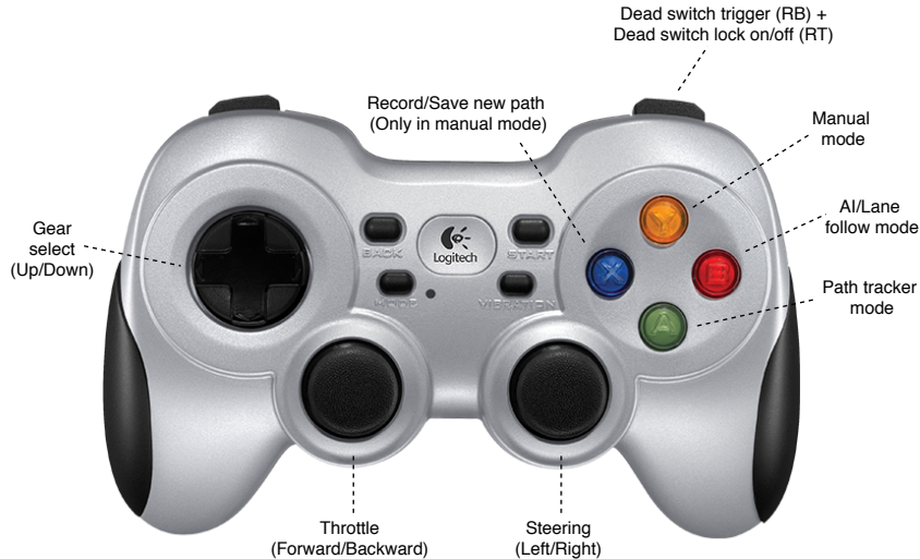
Figure 8.4: Overview of the joystick controls.
