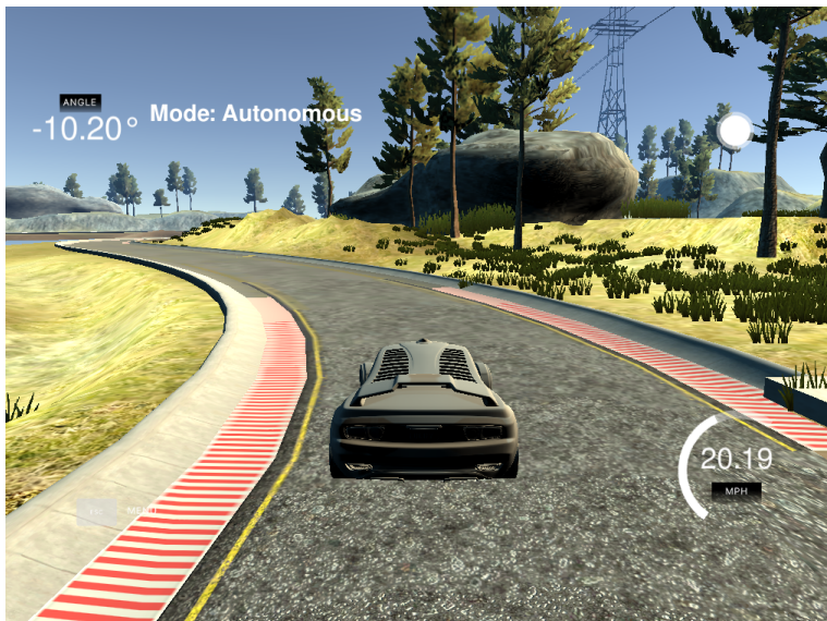
Figure 4.13: CNN controlling steering commands on the Udacity simulator.
