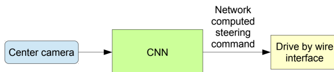
Figure 4.2: Block diagram of the Nvidia CNN steering control from a single camera. Ill: Nvidia
