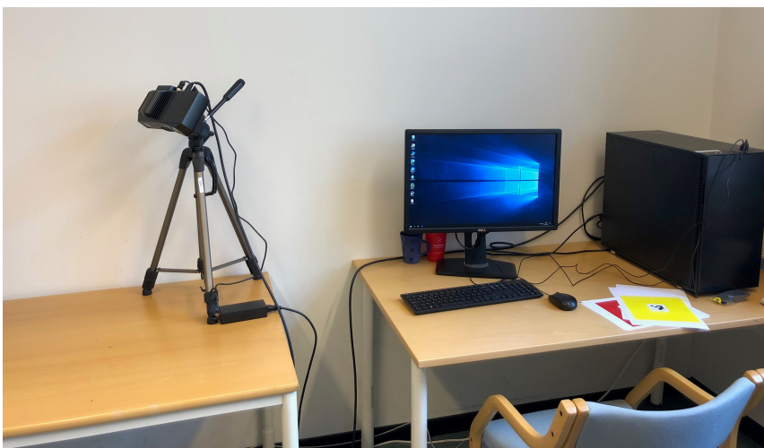
Figure 4.1: Image of the lab setup with Zivid camera on the left and the computer on the right.
