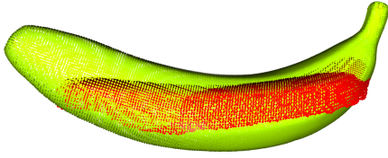
(a) translation error, error in [x, y, z] = [41.166, 19.693, 46.319] mm
