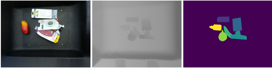
Figure 4.3: Example of WISDOM-Real dataset. Right: RGB image, middle: depth image, left: segmentation mask.
