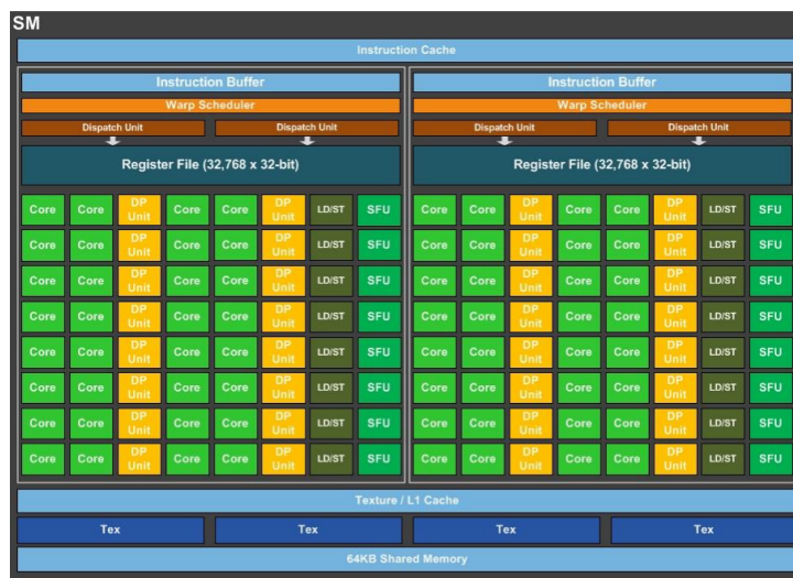
Figure 4: Block diagram of a streaming multiprocessor unit in the Pascal architecture [2]
