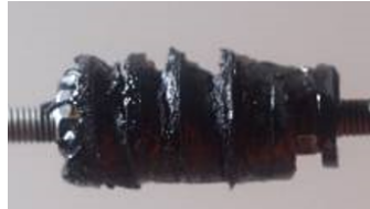
(b) Pigging of the test pipe not using CF.
