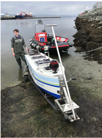
Figure 7.8: Place and method for launching and retracting ReVolt from the water. Here assisted by Andreas Bell Martinsen.
