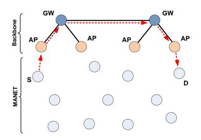
Figure 5.2: The concept of transit routing.
