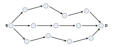
Figure 5.3: The concept of multipath load balancing
