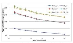
Figure 8. Aggregated throughput for mobile topologies with varying level of mobility (node velocity)
