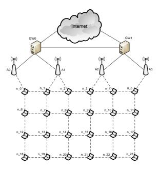
Figure 6.2: Example of a MANET interconnected with the global Internet through APs and GWs
