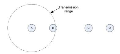
Figure 2.4: The hidden node and exposed node problems.
