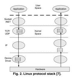
When a packet is received at an interface, it is put in a backlog queue. Then L3 processes it, and either forwards it out on an interface or pushes it up the stack to UDP or TCP. TCP has a receive queue to serve flow control.
