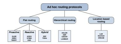
Figure 4.1: Classification of MANET routing protocols.
