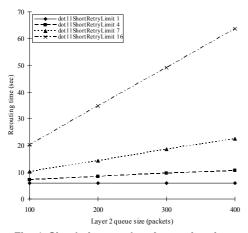
Fig. 4. Simulation results of rerouting time over layer 2 queue size.
