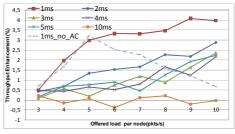
Figure 9. Throughput enhancement for mobile topologies
