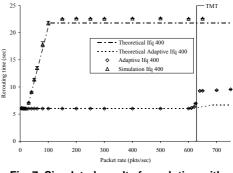
Fig. 7. Simulated results for solution with adaptive retry limit. (95% conf. int.)
