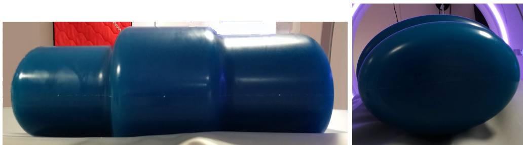
Figure 3.2: The ATCM phantom is elliptical with a small, large and medium section.
