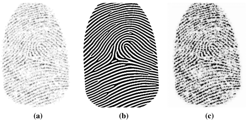
Figure 6.4: A fingerprint sample (6.4(a)) usually contains only a vague representation of the true present ridge structure (6.4(b)). An image enhancement can achieve a closer approximation (6.4(c)) of the true ridge structure from a sample.
