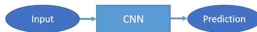
Figure 1.10: The workflow of a CNN is different to the one of the classical approach (compare to Figure 1.1). CNNs do not clearly split feature extraction and decision making. This allows to train a feature extraction, which is helpful for solving the actual task.
