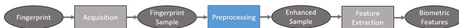
Figure 3.2: Preprocessing of fingerprint samples can be part of the workflow. Preprocessing can be used for an enhancement of a sample with respect to its biometric quality. An enhanced sample may have a higher biometric utility.
