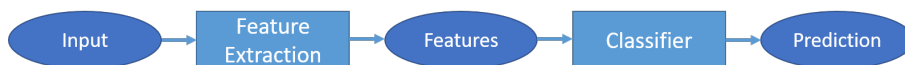
Figure 1.1: In the classical workflow of pattern recognition, features are extracted by a feature extraction process first. A classifier predicts from these features.
