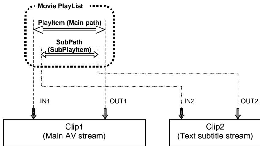
Figure 3-5 - An example of Main path and Sub path structure with Text subtitle presentation path
