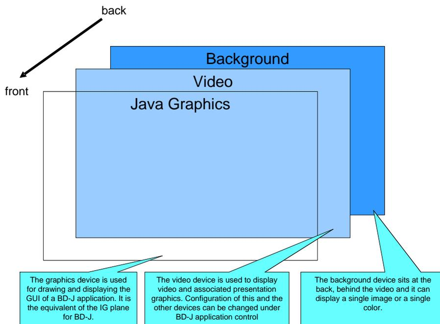
**Figure 6-2 – BD-J system device model**
