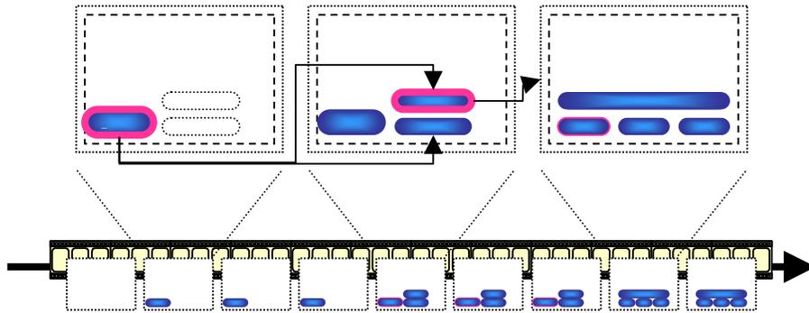
Figure 5-12 – Example of Multi-page Menu with dynamic Button display
