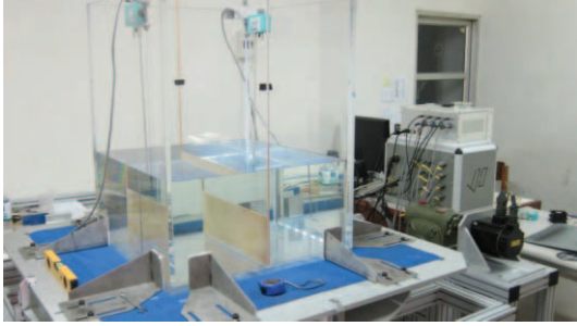
FIGURE 2: Photograph of the experiment setup of a baffled tank.
