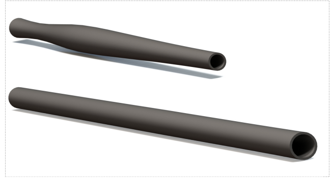
Figure 7: Three-dimensional of the reference reactor (bottom) and of the (D,L)-optimal reactor (top).
