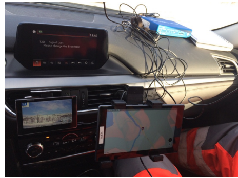
Figure 4.8: Video logger and C-ITS equipment inside the vehicle during test runs.
