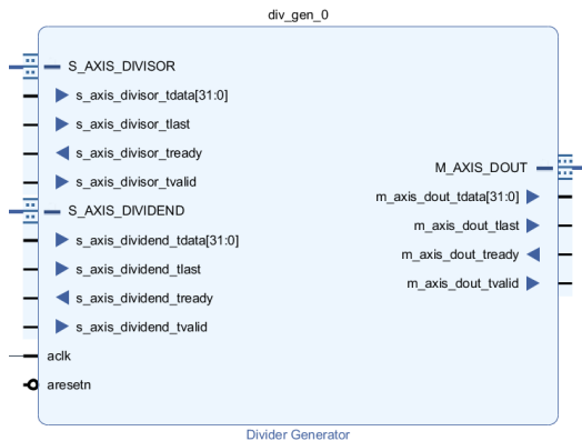
Figure 2.10: Generated Divider Block in Xilinx Vivado
