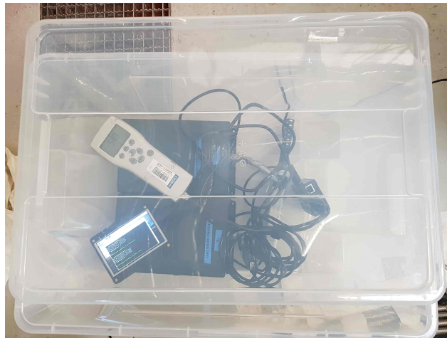
Figure 5.1: Calibration of CO 2 sensors in semi-enclosed box.
