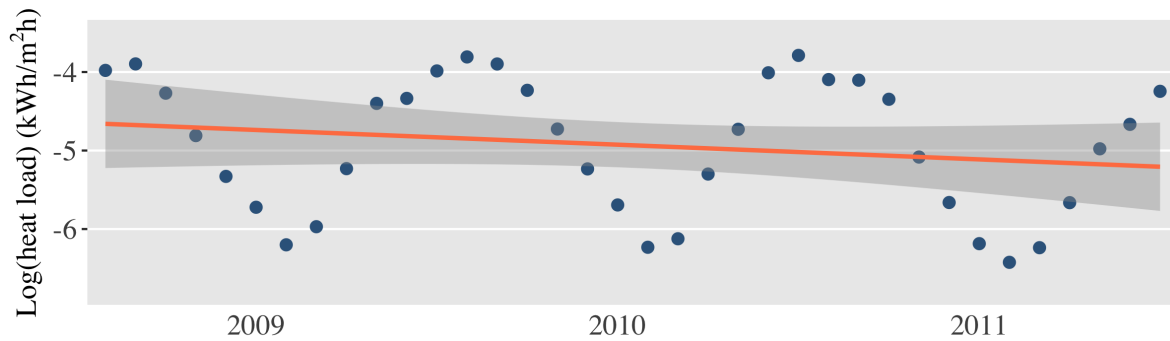
Figure 2.7: Mean monthly values of heat consumption (blue dots) in Trondheim for each month. The red line shows the best linear model for the consumption, and shaded area denotes the 95% confidence interval.
