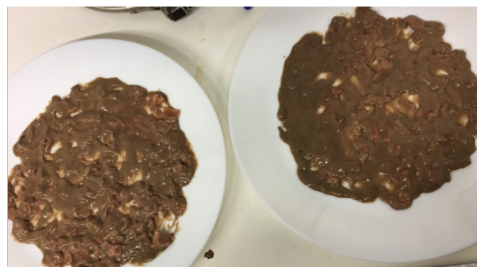
Figure 11: Fat-reduced sediment from salmon intestines spread on plates before drying in oven at 50°C and 100°C.
