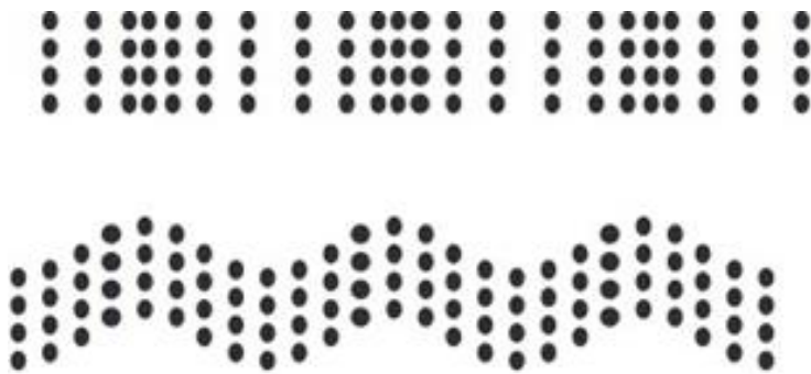
Figure 11: Illustration of the particle movement association with longitudinal waves (top) and shear waves (bottom) (O'Brien Jr 2007).
