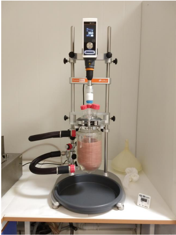
Figure 18: The figure illustrates the enzymatic hydrolysis set-up used in the present work during experimental trials.
