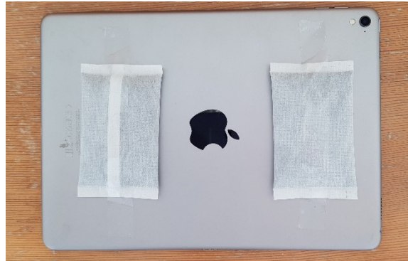
Figure 12: Heating pads as heating source attached to the iPad
