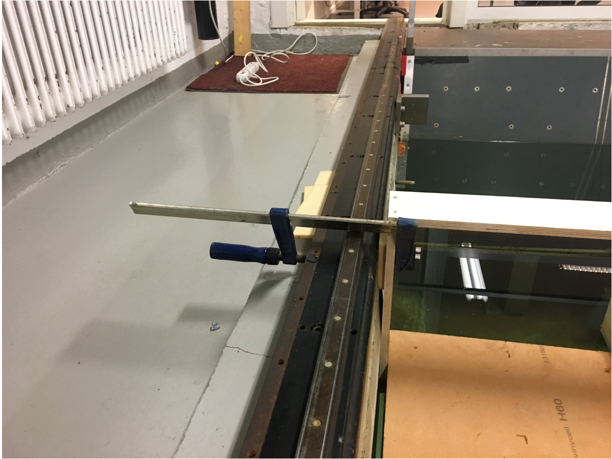
Figure 5.8: Forcing tool fastening the dock to the side of the basin
