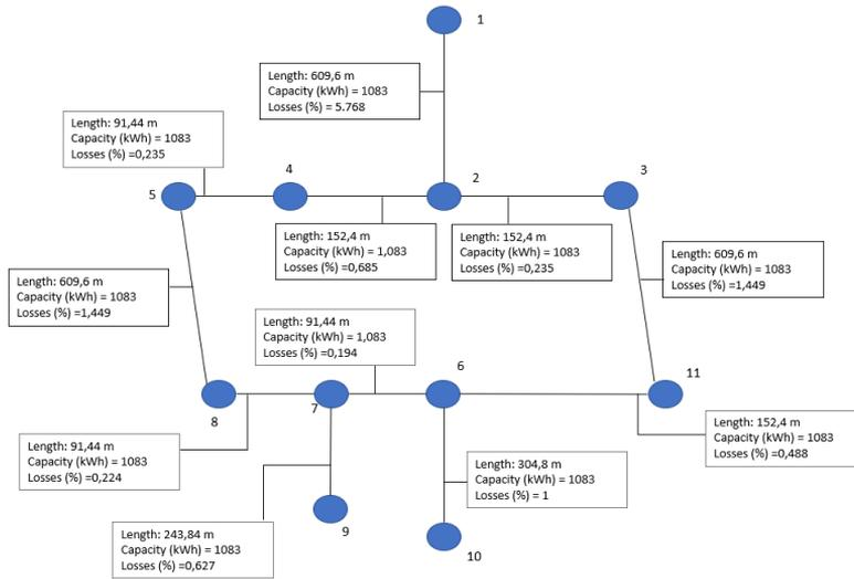
**Figure 6.2:** Grid properties for Loop structure
