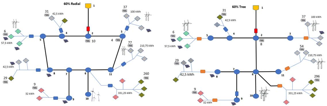
**Figure 6.10:** Battery placement and capacity 60 % RES both topology
