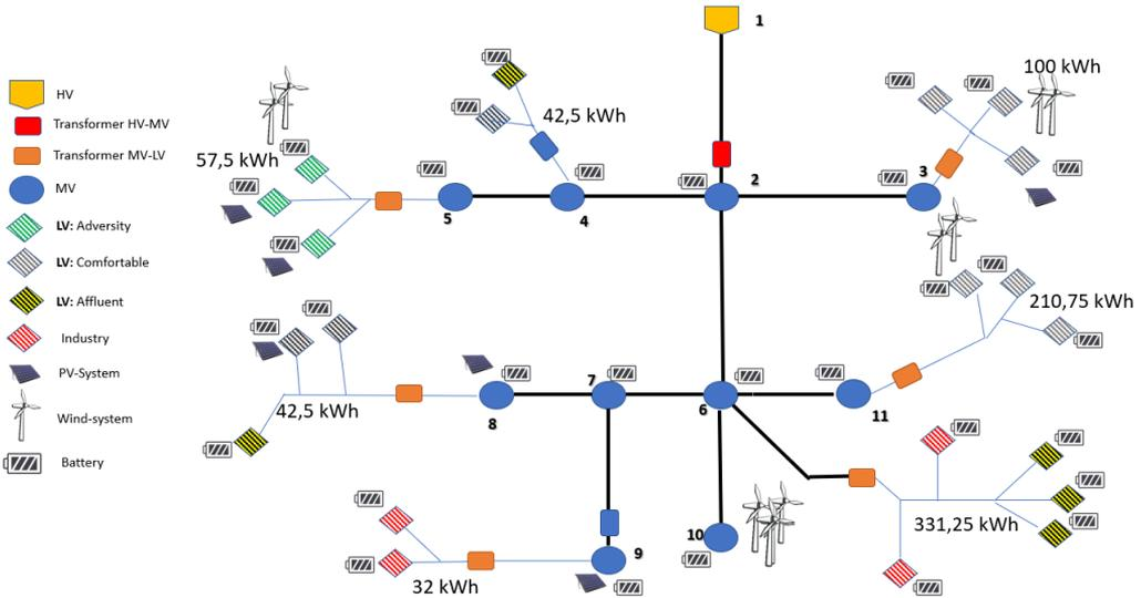
Figure 5.3: The model with Radial Tree topology
