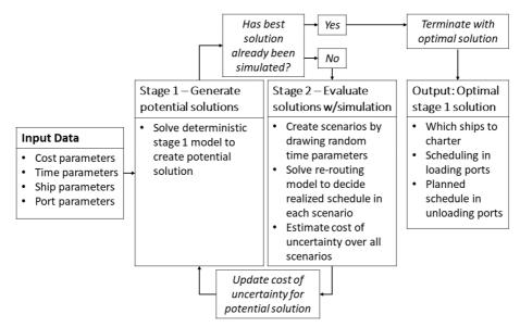
Figure 5.1: Flow chart of the optimization-simulation framework
