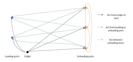
Figure 5.2: Illustration of original network structure
