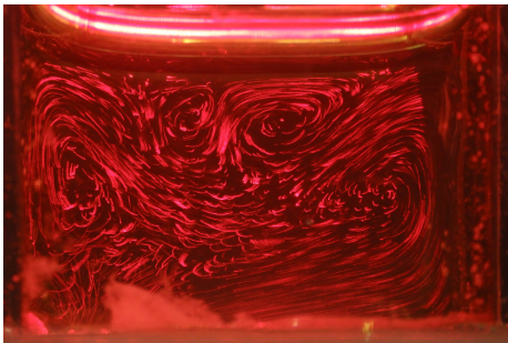
(e) E = 200 \text{ V mm}^{-1} , 35 s after initiation. T \approx 95 \text{ }^\circ\text{C} .
