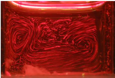
(c) E = 200 \text{ V mm}^{-1} , 15 s after initiation. T \approx 95 \text{ }^\circ\text{C} .
