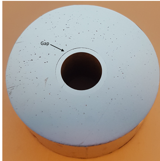
Figure 15: Surface of Sample 4, with a visible gap between the insert and cast aluminium.
