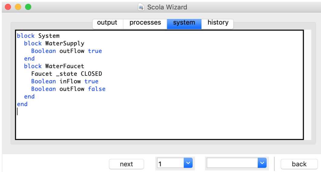
Figure 3.8: System window in ScOLA Wizard. It shows the whole system and its components, represented by blocks.
