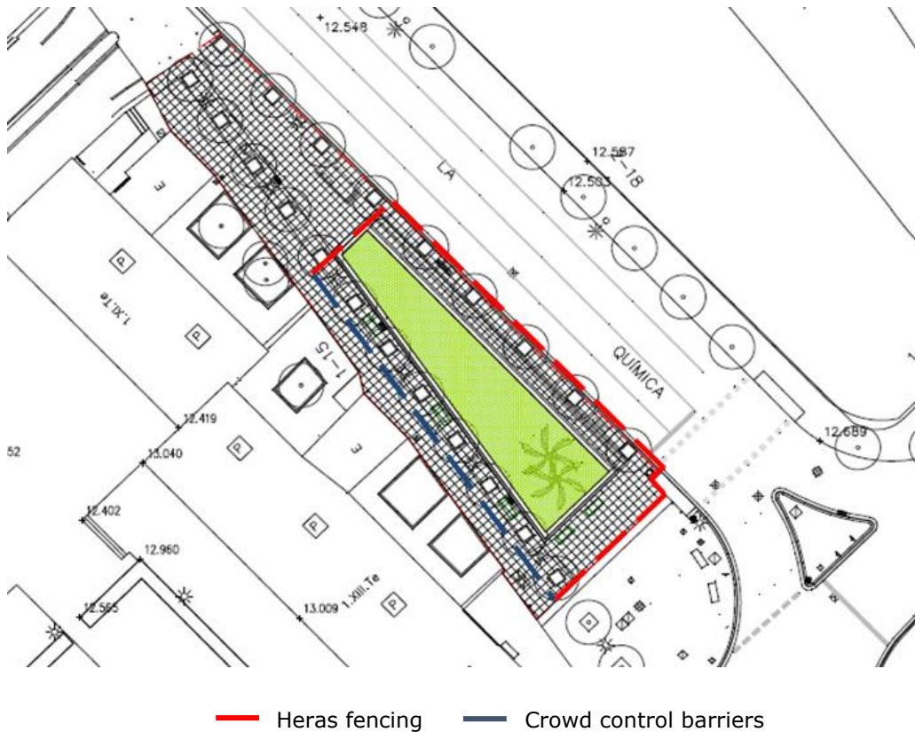
Figure 4.9: Perimeter fence in Carrer Química (1 st phase) (Civil Stone)
