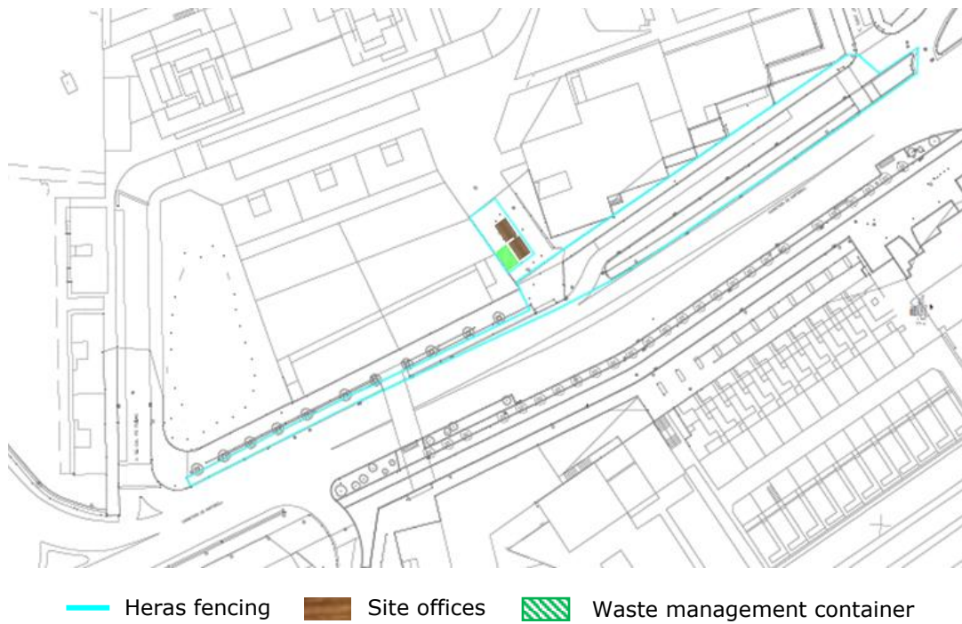
Figure 4.23: Final proposal of the storage area by the CM (Civil Stone)
