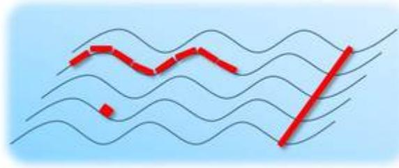
**Figure 1.2:** A schematic of three WEC types: a point absorber (bottom left), an attenuator (top left) and a terminator (right) [10]
