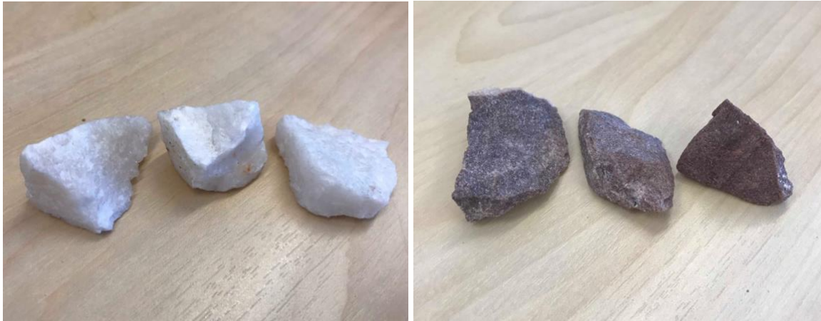
Figure 3.6 Samples of two of the quartz types used in the rapid heating experiments. Mass of the samples is 15 \pm 5 g.
