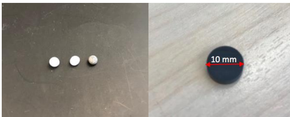
(a) Samples of the three different quartzes after heat treatment. (b) Graphite substrate with diameter and height of 10 mm and 3 mm, respectively.
