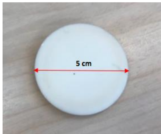
Figure 3.7 Alumina substrate, with diameter of 5 cm and height of 0,5 cm, used in the rapid heating experiments.
