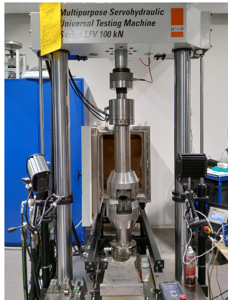
(b) Walter + Bai Universal Testing Machine, used for tensile testing of wire samples.
