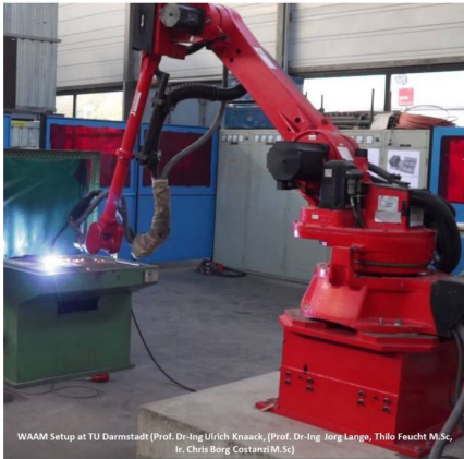
(a) Image taken during a wire arc additive manufacturing (WAAM) experiment at Technische Universität Darmstadt, showing a typical WAAM-setup. From [72].
