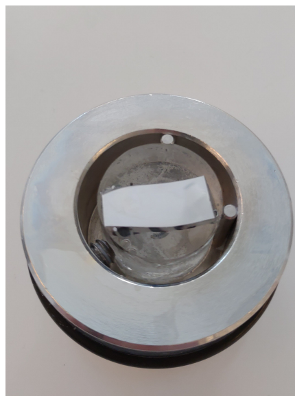
(b) Sample holder for vibration polishing, weighing 400 g, containing a longitudinal 4043 single flight-wire sample.
