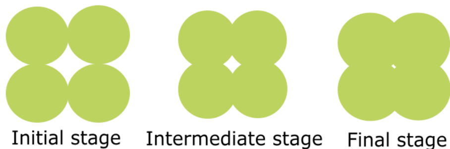
Figure 2.6: An illustration of the three sintering stages. In the initial stage the particles rearrange and necks start to form. In the intermediate stage the pores size is reduced with diffusion and shrinkage occurs. In the final stage the porosity is closed and pores are removed by vacancy diffusion and grain boundary movement.
