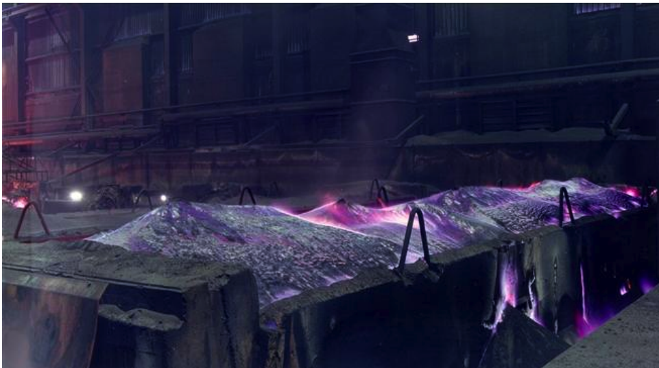
Figure 2.3: The characteristic blue flame of the Acheson furnace, a result of carbon monoxide burn-off [16].
