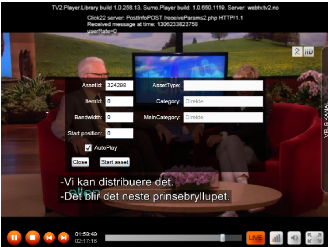
Figure 6.15: This screen capture presents the TV2 Sumo service running our information gathering code in the background. We can see the KP response to the client saying that it's the Click22 server and that the message was received at a given time stamp. The userRate parameter is used in the application controlled client described in section 5.2
